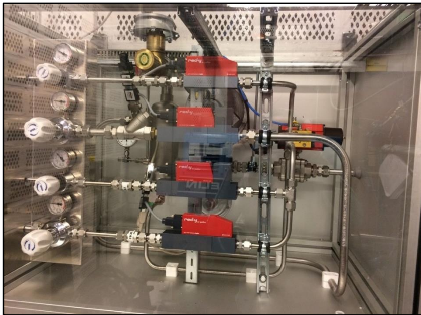
Figure 2: Fuel mixture control system.
