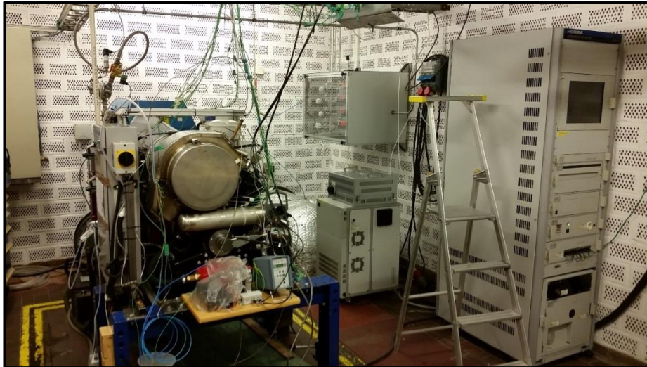
Figure 1: GasBox equipped with temperature and pressure sensors, and a gas analysis system.
